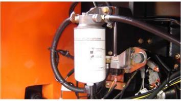
Lube Point(s) - Replaceable Element Interval - Drain water daily; Change every year or 600 hours of operation
