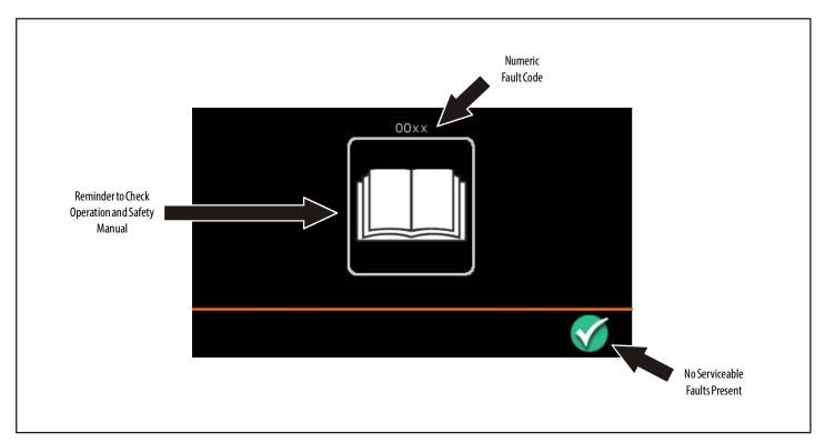
Figure 5-11. Operational Fault - No Graphics Screen
