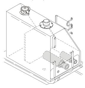
Lube Point(s) - 2 Interval - Every 2 years or 1200 hours of operation. Remove and clean at time of hydraulic oil change.
