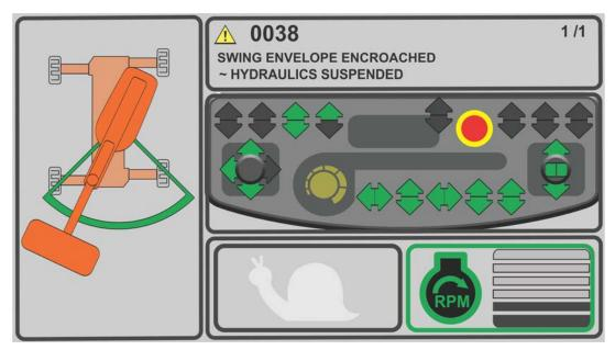
Figure 5-34. Swing DTC Screen
