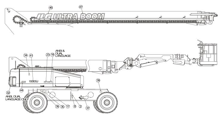
Figure 4-13. Decal Location Sheet 6 of 6
