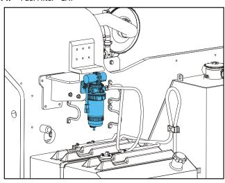
Lube Point(s) - Replaceable Element Interval - Drain water daily; Change every year or 600 hours of operation
