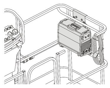
SkyWelder<sup>™</sup> is capable of TIG and Stick welding, producing 200 Amps at 100% duty cycle or 250 Amps at 50% duty cycle. It receives power from the SkyPower<sup>™</sup> system.
