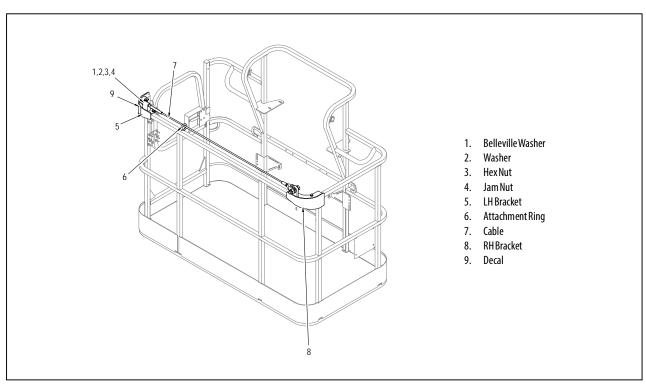
Figure 7-2. Bolt On Fall Arrest System
