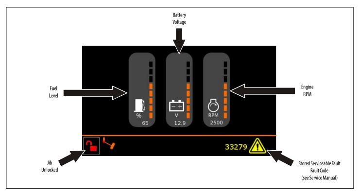
Figure 5-8. Serviceable Fault Screen
