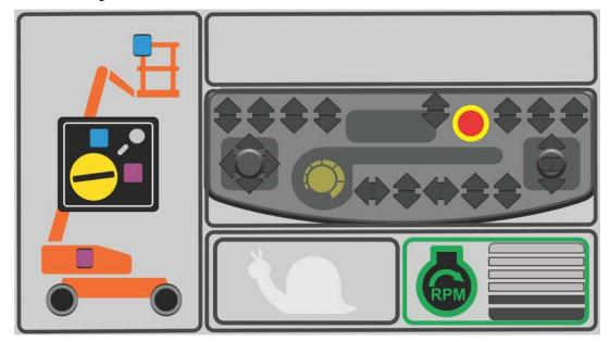
Figure 5-24. Keyswitch In Ground Mode Screen
