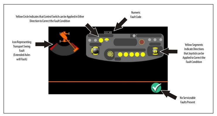
Figure 5-15. Transport Swing Fault Screen
