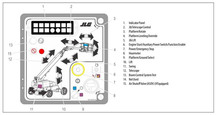
Figure 3-1. Ground Control Station
