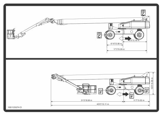
Figure 4-7. Lifting and Tie Down Chart
