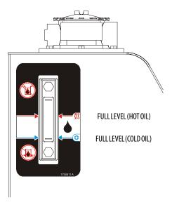
Lube Point(s) - Fill Cap Capacity - Standard 31 gallons (117 liters) Optional 52.8 gallons (200 liters)
