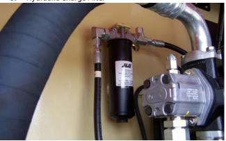
Lube Point(s) - Replaceable Element Interval - Change after first 50 hours and every 300 hours thereafter or as indicated by condition indicator.
