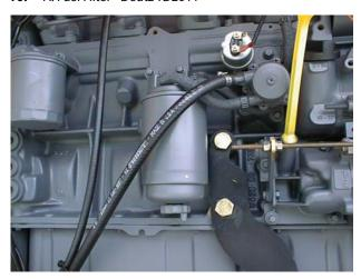
Lube Point(s) - Replaceable Element Interval - Every year or 600 hours of operation
