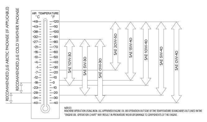
**Figure 8-2. Engine Operating Temperature Specifications**
