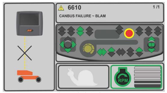
Figure 5-26. CAN Bus Lost Screen
