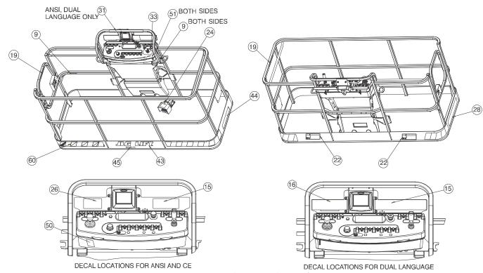
Figure 4-9. Decal Location Sheet 2 of 6
