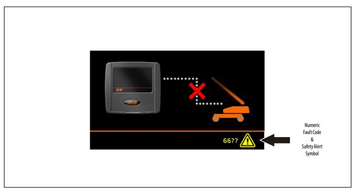
Figure 5-7. CAN Communication Error Screen
