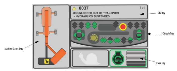
Figure 5-23. Machine Operating Screen
