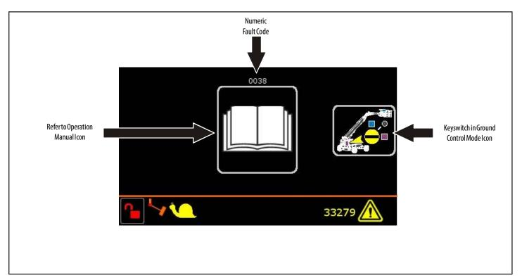
Figure 5-10. Keyswitch in Ground Control Mode with Operational Faults
