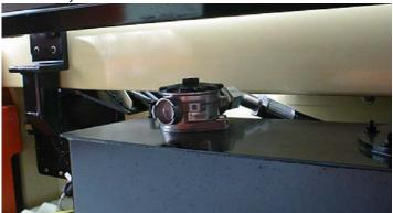
Lube Point(s) - Replaceable Element Interval - Change after first 50 hours and every 300 hours thereafter or as indicated by condition indicator
