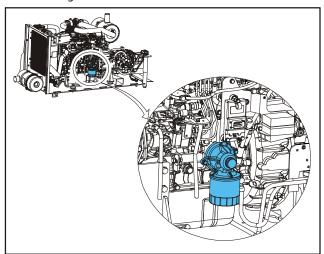
Lube Point(s) - Fill Cap/Spin-on Element
