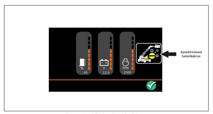
Figure 5-9. Keyswitch in Ground Control Mode Screen
