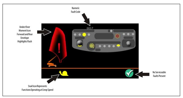
Figure 5-18. Over/Under Moment Fault Screen
