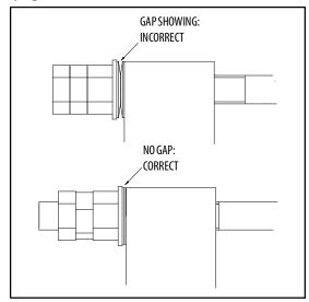
Figure 7-1. Bolt-On External Fall Arrest Cable Tension
