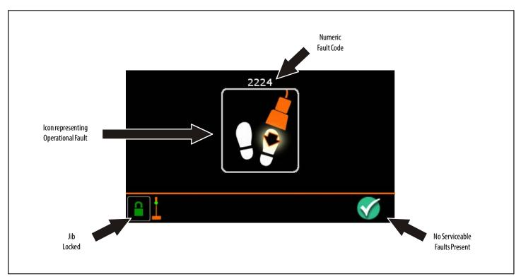
Figure 5-12. Operational Fault - With Graphics Screen
