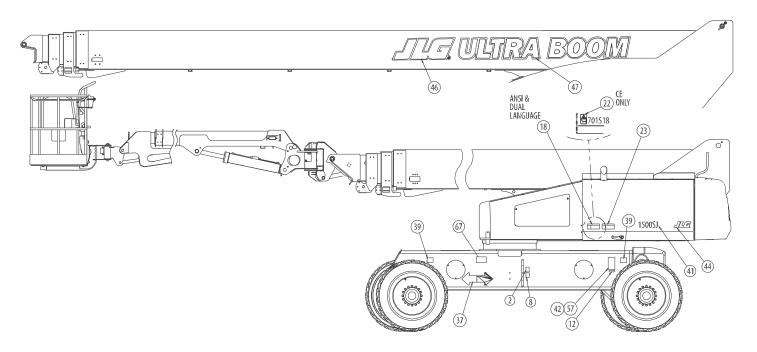
Figure 4-8. Decal Location Sheet 1 of 6
