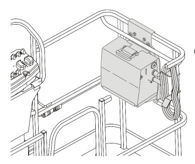
SkyCutter™ is capable of cutting up to a thickness of 3/8" metal. It can produce 27 A at 92 VDC at 35% duty cycle or 14 A at 92 VDC at 60% duty cycle. This accessory receives power from the Sky-Power™ system.
