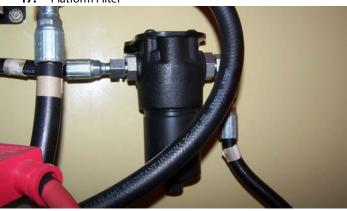
Lube Point(s) - Replaceable Element Interval - Change after first 50 hours and then every year or 600 hours of operation thereafter
