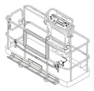
SkyGlazier™ allows glaziers to position panels efficiently. The glazier package consists of a tray that attaches the bottom of the platform. The panel rests on the tray and against top-rail of the platform, which is padded to prevent damage. SkyGlazier™ includes a strap to secure the panel to the platform rail.
