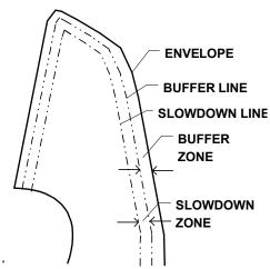
When the platform approaches the edges of the operating envelope all machine functions are slowed down except jib and platform functions, telescope in or out at the rearward edge and telescope in or out on the forward edge are slowed down automatically by the boom control system to reduce machine motions.
