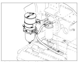
Lube Point(s) - Replaceable Element Interval - Drain water daily; Change every year or 600 hours of operation
