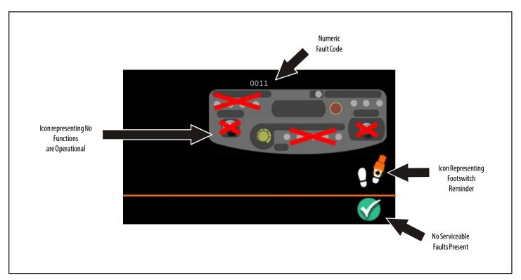
Figure 5-13. Operational Fault - Footswitch Open Screen
