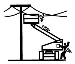
• Maintain distance from electrical lines, apparatus, or any energized (exposed or insulated) parts according to the Minimum Approach Distance (MAD) as shown in Table 1-1.
