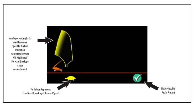
Figure 5-16. Backward Envelope Speed Reduction Fault Screen
