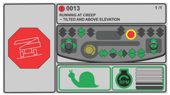
Figure 5-39. Machine Tilted Mode Screen
