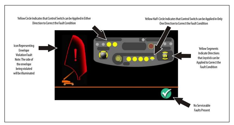
Figure 5-17. Forward Envelope Violation Fault Screen
