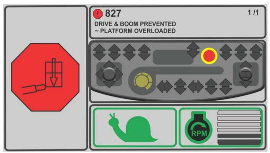
Figure 5-32. Overload DTC Screen
