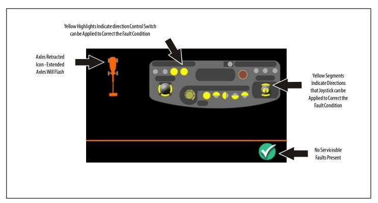
Figure 5-14. Out of Transport - Axles Retracted Screen
