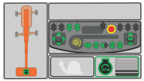
Figure 5-36. Jib Locked Screen
