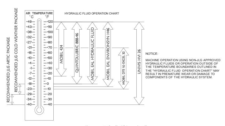
Figure 8-3. Hydraulic Oil Operation Chart
